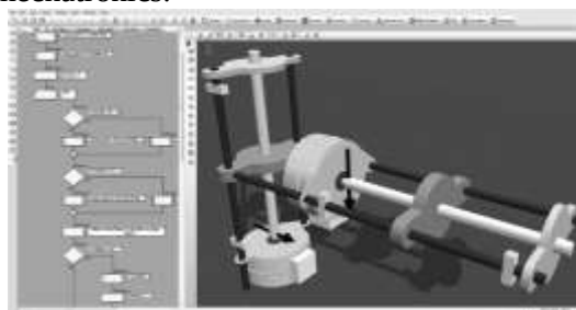
Fig. 1 Electromechanical components example in Flowcode
