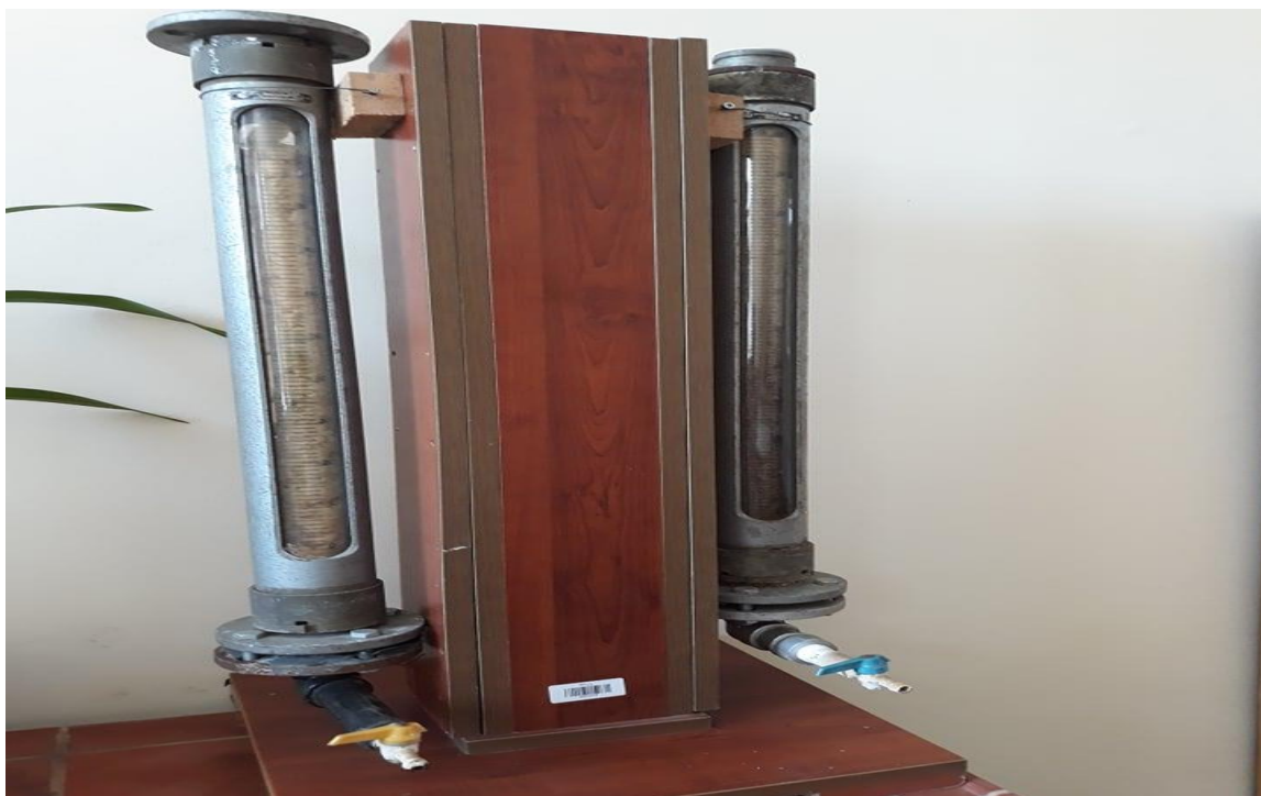
Picture 20. Seawater purification in different sorbents (polyurethane foam - on the left, sawdust - on the right)
