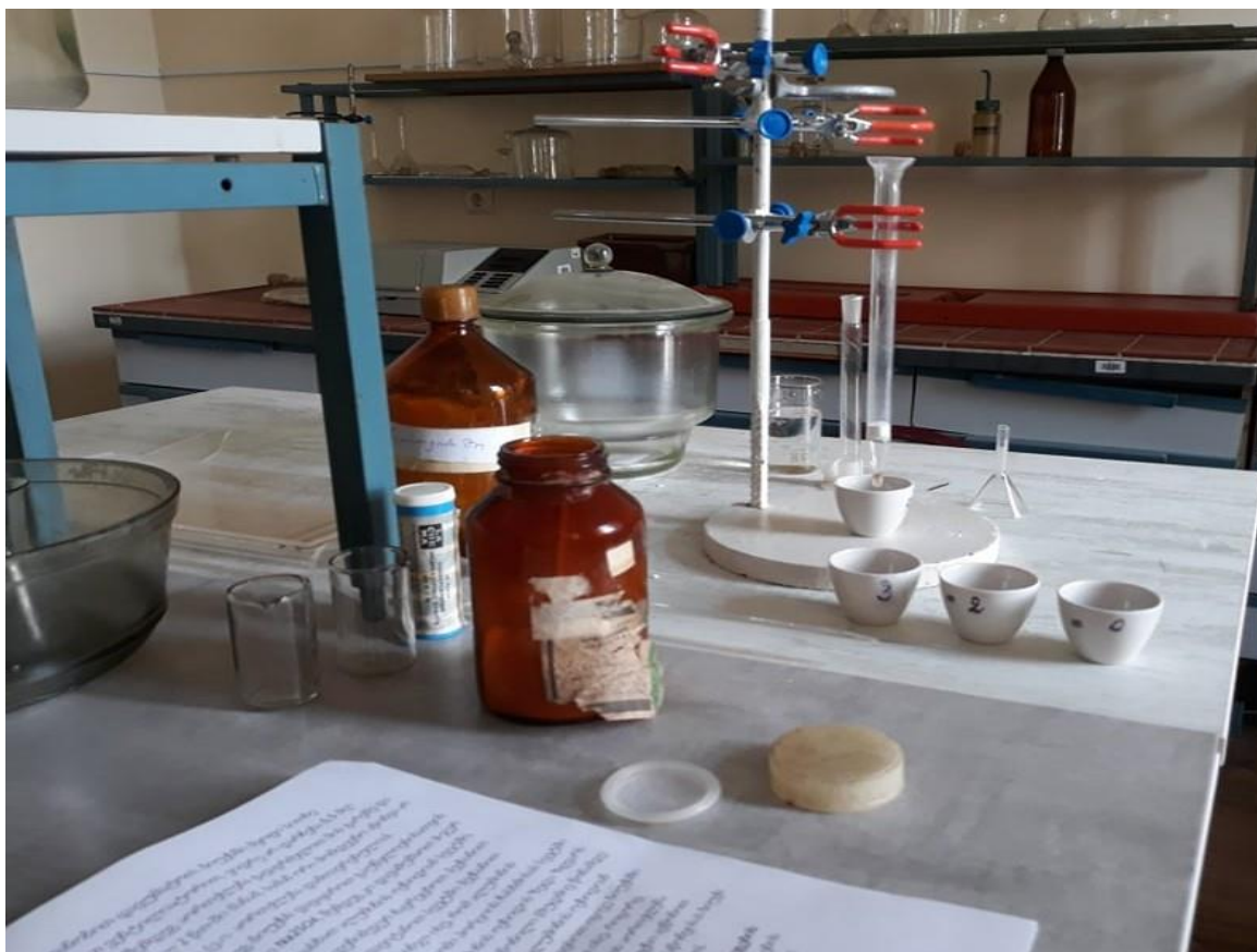
Picture 21. Preparation of sorbent columns and extract filtration process in \text{Al}_2\text{O}_3 sorbent column, for polar compound sorption: Column length– 20 cm, \text{Al}_2\text{O}_3 – 4-6cm, n-hexane - 6-10 ml
